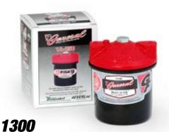
1A-25B 3/8" General Fuel Oil Filter 10 GPH Firing Rate at 10 Microns 40 PSI
